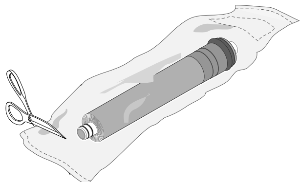
Figure 8: Cut the membrane bag at the end of the membrane with the 2 O-Rings. Do not damage or touch the membrane!
